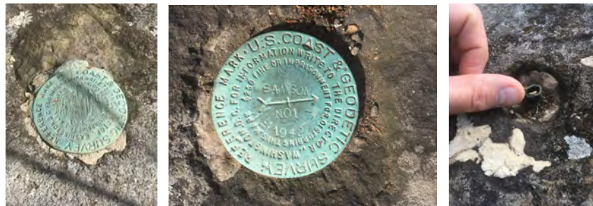
Markers from the 1942 U.S. Coast and Geodetic Survey on the summit of High Point. The left and middle are reference markers whose arrows point to the triangulation station marker. The right-most photo shows the location which once held the 1942 and 1970 triangulation station markers, which were stolen, and now only the metal stem remains.
